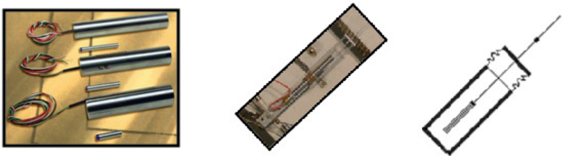
Figure 7.8. General views of LVDTs [50]
