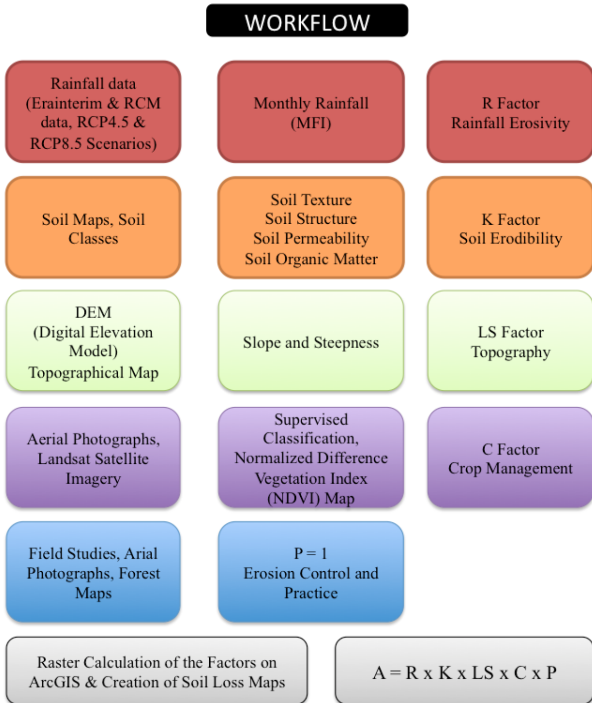
Figure 3.3. A Schematic Approach to the Workflow of the RUSLE Model.
