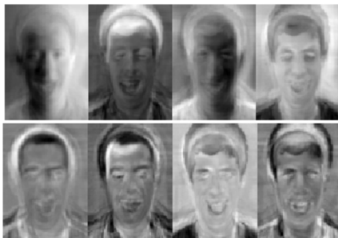
Figure 1.2. Sample eigenfaces (top row) showing the tendency of the principal components to capture major variations such as lighting direction and their corresponding fisherfaces (bottom row) showing the ability to discount those factors unrelated to classification [2].
