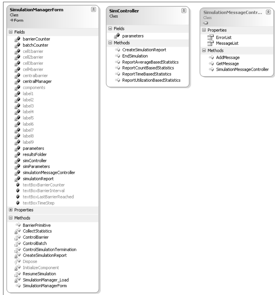
Figure F.5. SimulationManager and its sub-components class diagrams
