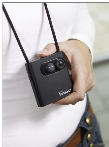
Figure 2.1. SenseCam [17]. A sensor augmented wearable camera that captures photographs periodically or when it is triggered by a sensor.
