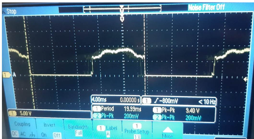
Figure 5.9. The beam current results measured at 20 kV using the Faraday cup connected to an oscilloscope.
