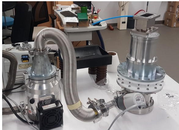
Figure 5.1. Plasma chamber vacuum test using turbomolecular vacuum pump.
