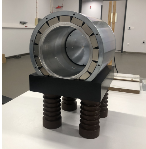
Figure 3.39. The system after the permanent magnets are placed between the aluminum part and the ST37 iron.
