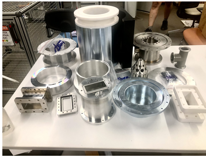
Figure 3.38. The PM-MDIS components, including the plasma chamber and the dual electrode extraction system are shown before assembly.
