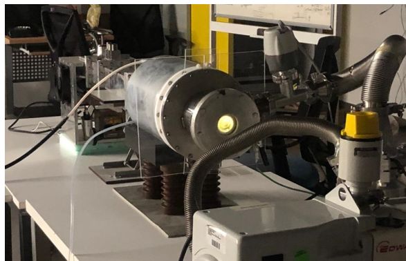
Figure 5.4. Beam visible through fluorescent screen placed at the end of the operating PM-MDIS.
