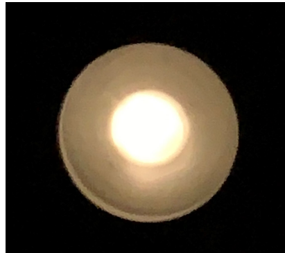
Figure 5.8. The beam image from the fluorescent screen at the end of the LEBT line.
