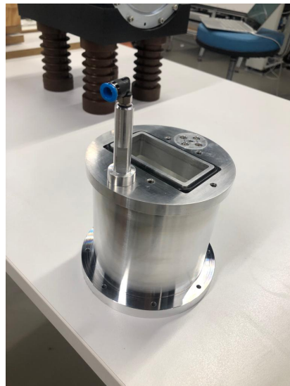
Figure 3.40. Produced plasma chamber including vacuum window and gas entrance pipe.
