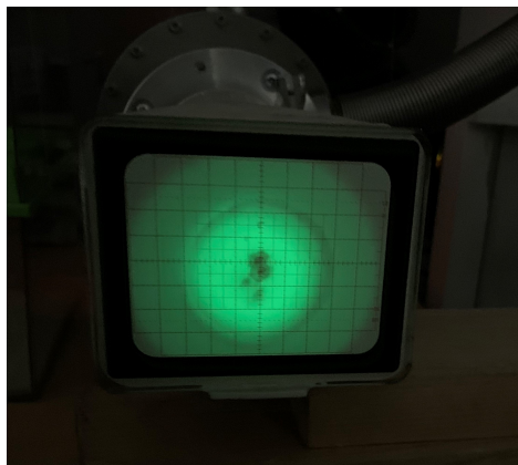
Figure 5.5. The obtained beam image from the fluorescent screen placed at the end of the PM-MDIS system.
