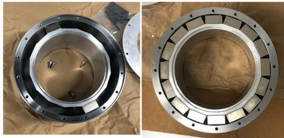
Figure 3.30. The produced trial component before and after the permanent magnets are placed.
