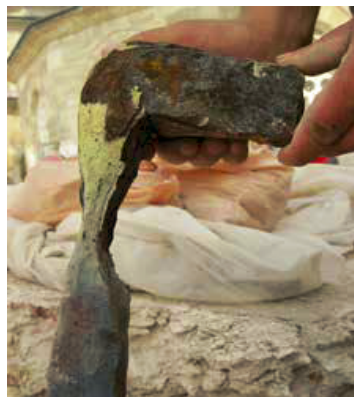
Figure 2.6. The old peripheral tie beam
