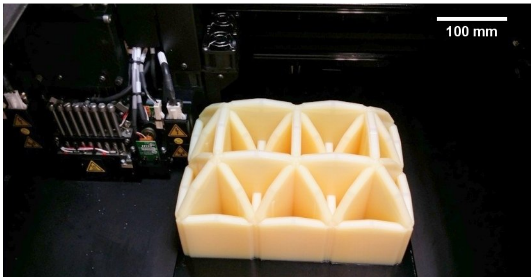
Figure 6.1. Manufacturing of the octahedron structure with 3D printer.
