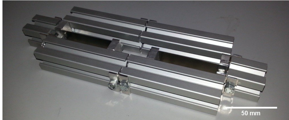
Figure 6.9. The prototype of the inertial amplification mechanism with ultra wide band gap.
