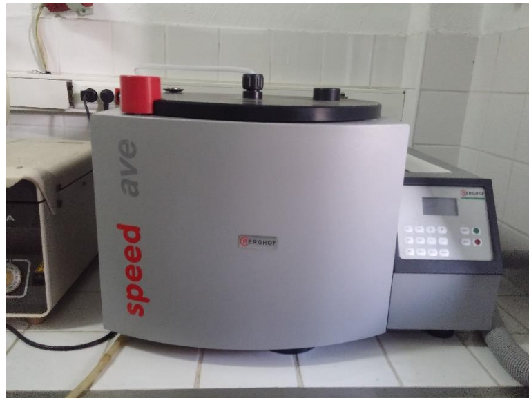
Figure 3.2. The microwave equipment used in the study (Berghof Speedway MWS+3).
