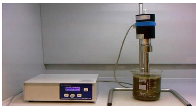
Figure 3.1. The ultrasonic homogenizer (Bandelin-Sonopuls HD 3400).
