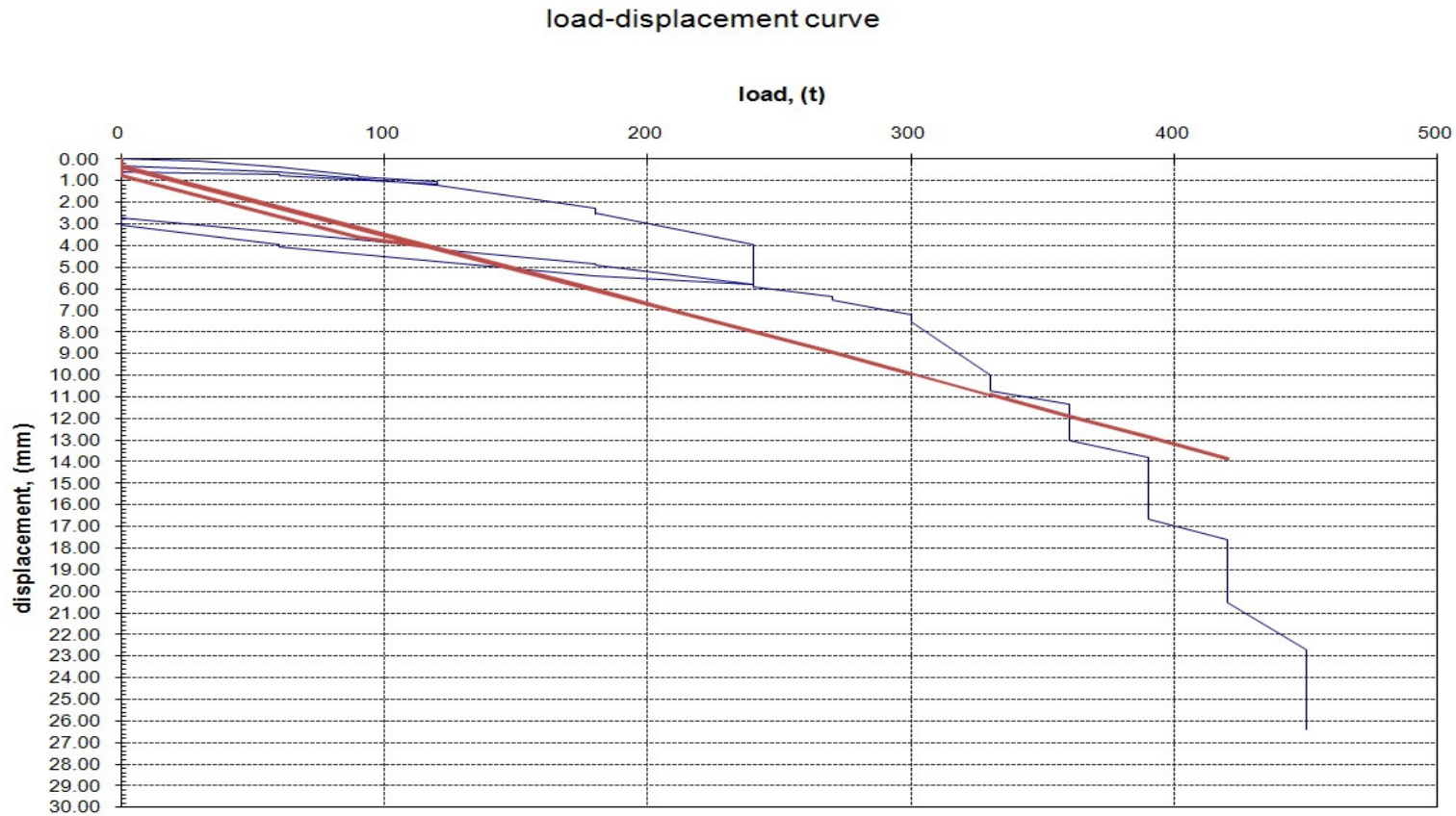
Figure 3.64. Site measured(blue) and numerically simulated(red) load versus displacement curve of case4.
