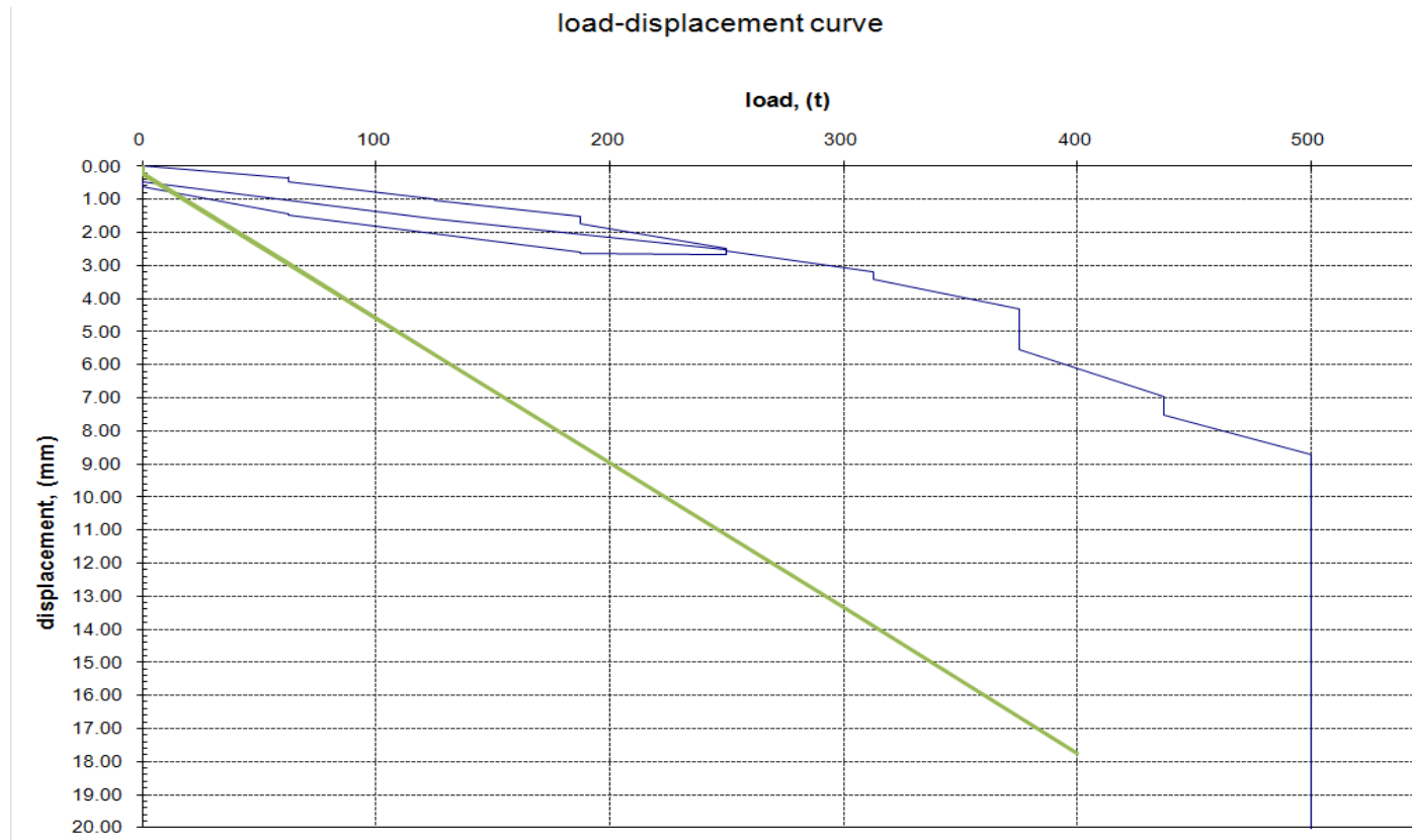
Figure 3.10. Site measured(blue) and numerically simulated (green) load versus displacement curve of case 1.
