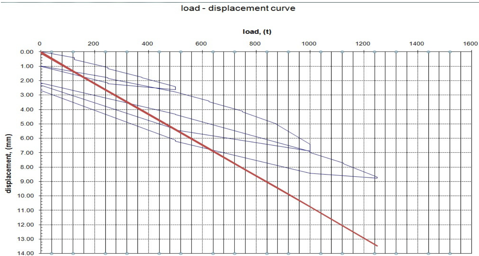
Figure 3.75. Site measured(blue) and numerically simulated(red) load versus displacement curve of case5.
