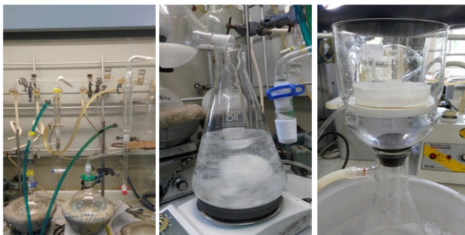
Figure 3.1. a) Synthesis, b) Precipitation and c) Washing of SEBS-g-PEO.
