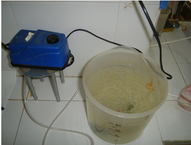
Figure 4.3 Batch reactor used to enrich the microorganisms in Ömerli water
