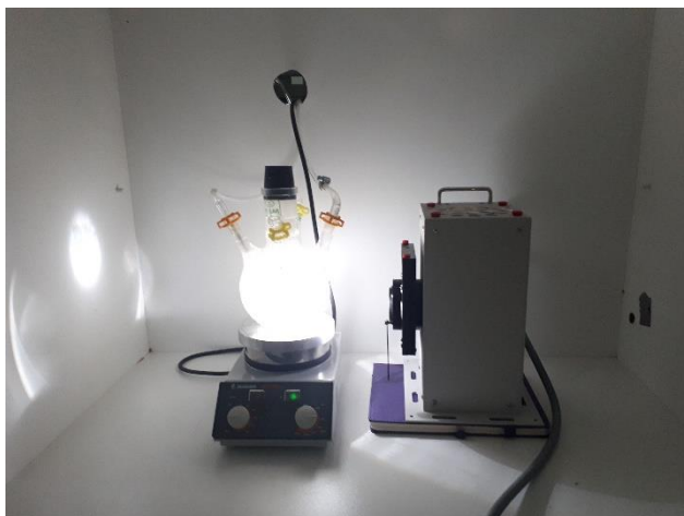
Figure 3.5. The setup of photocatalytic water splitting.
