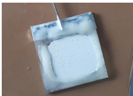
Figure 3.1. Un-doped \text{SrTiO}_3 prepared by SSR, coated by doctor blade.
