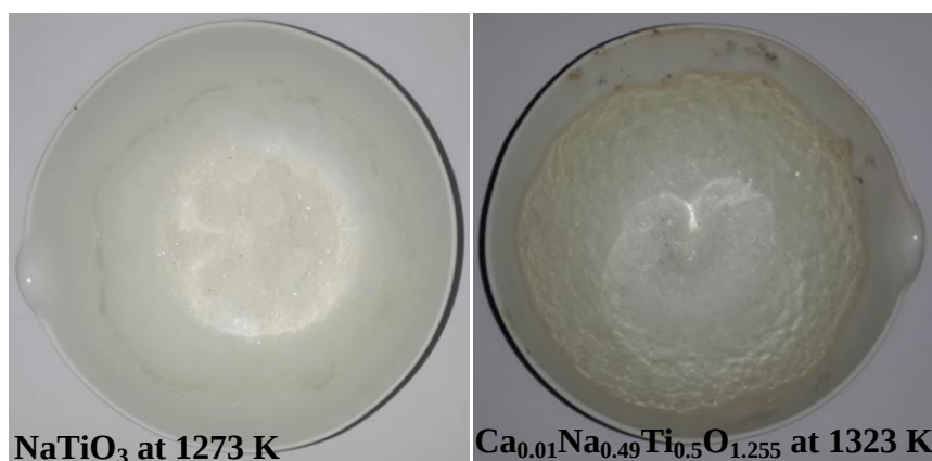
Figure 4.1. Burned and stuck \text{NaTiO}_3 and \text{Ca}_{0.01}\text{Na}_{0.49}\text{Ti}_{0.5}\text{O}_{1.255} samples in the crucible.
