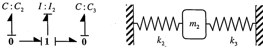
Figure 3.15. High frequency oscillation mode of case 2
