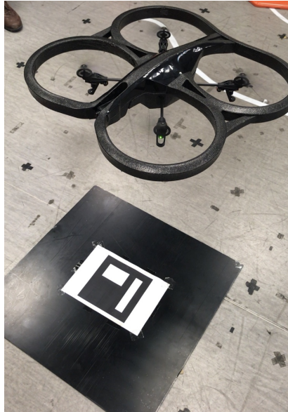
Figure 5.4. AR.Drone hovering over ArUco marker
