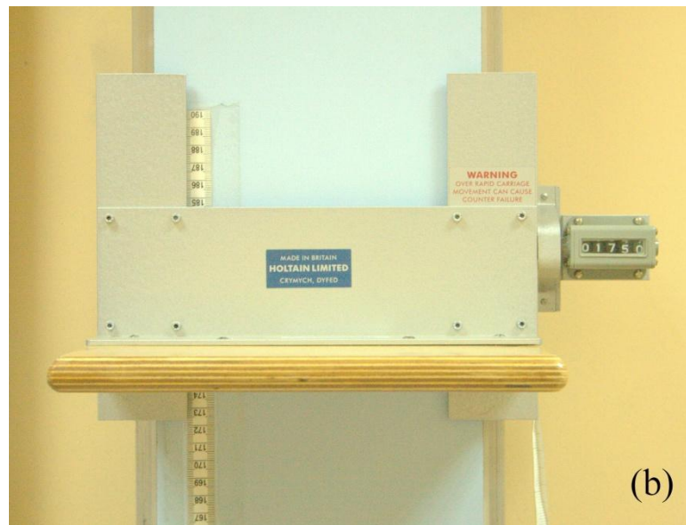
Figure 4.11. Stadiometer (a) Front view (b) Indicator (Cont.).
