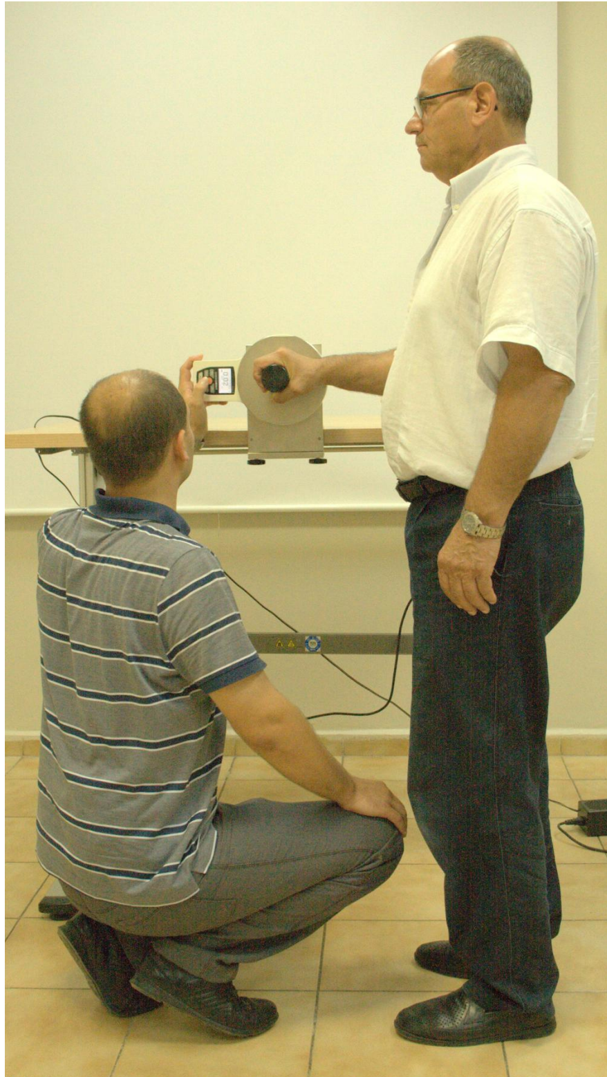
Figure 4.27. Measurement of hand torque strength while standing (cylinder).
