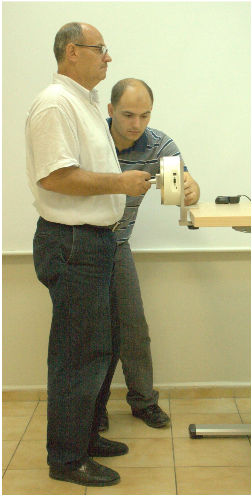
Figure 4.28. Measurement of hand torque strength while standing (Ellipsoid, circular, key).
