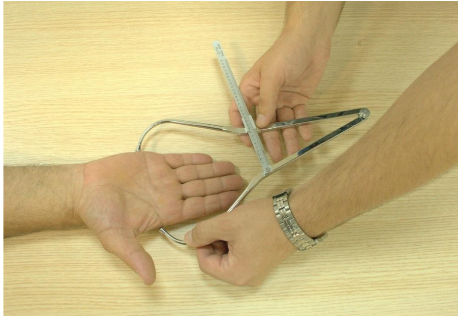
Figure 4.21. Measurement of hand breadth with sliding caliper.
