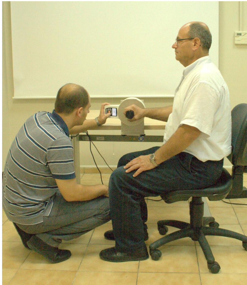
Figure 4.25. Measurement of hand torque strength while sitting (cylindrical).
