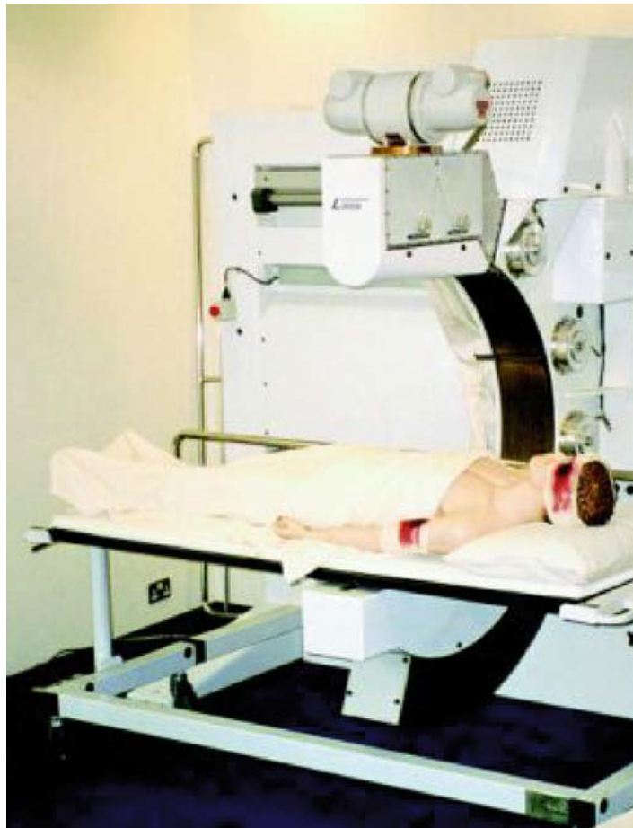
Figure 3.3 Lodox Statscan on a trauma patient. System is mounted on the wall, movement is on one direction [13].
