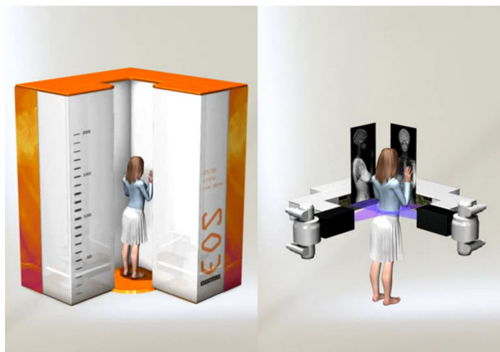
Figure 3.2 EOS system designed for 2D and 3D image acquisitions, system detector and X-ray source parts are vertically moving to get a biplaner digital images [12].
