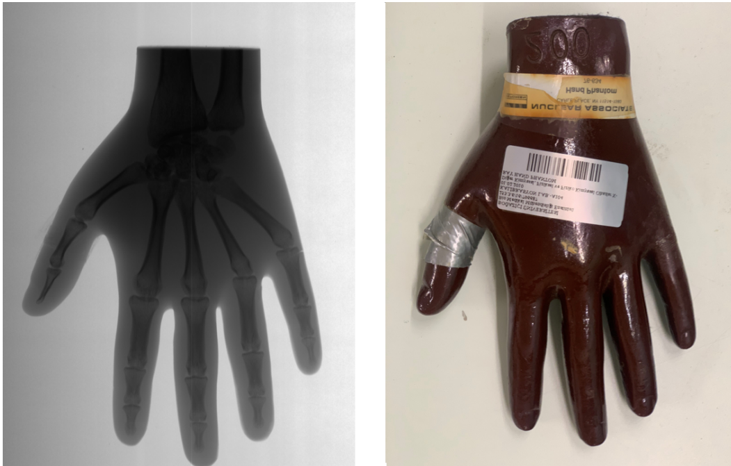
Figure 2.12 Victoreen Nuclear Associate Hand Phantom 76-634 x-ray image taken by SyncBox controlled TDI detector x-ray scanner. 0.5 mm aluminum filtration has been used. Exposure parameters are 60 kVp, 10 mA duration 1.8 sec. Total image acquisition time 5 seconds.
