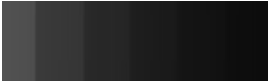
Figure 3.16 Contrast phantom image output after the calibration of TDI detector frequency, motor system calibration, and X-ray parameters optimization.
