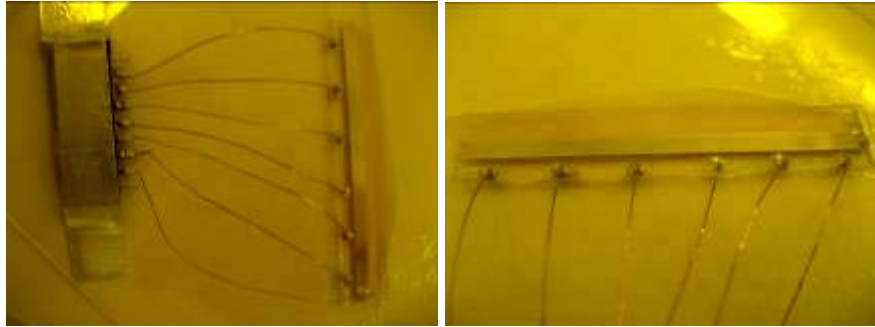
Figure 2.30. Wired and encapsulated PLED samples
