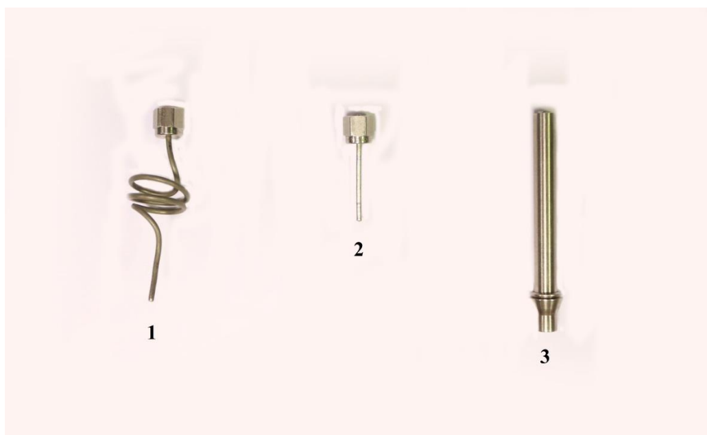
Figure 3.3. Different Configurations to Introduce Liquid Reactant Mixture into Furnace: 1. 1/16" spiral-shaped. 2. 1/16" straight. 3. 1/4" straight.
