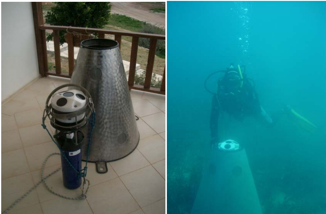
Figure 3.12. Acoustic wave & current meter (AWAC) and its protective frame before and after deployment
