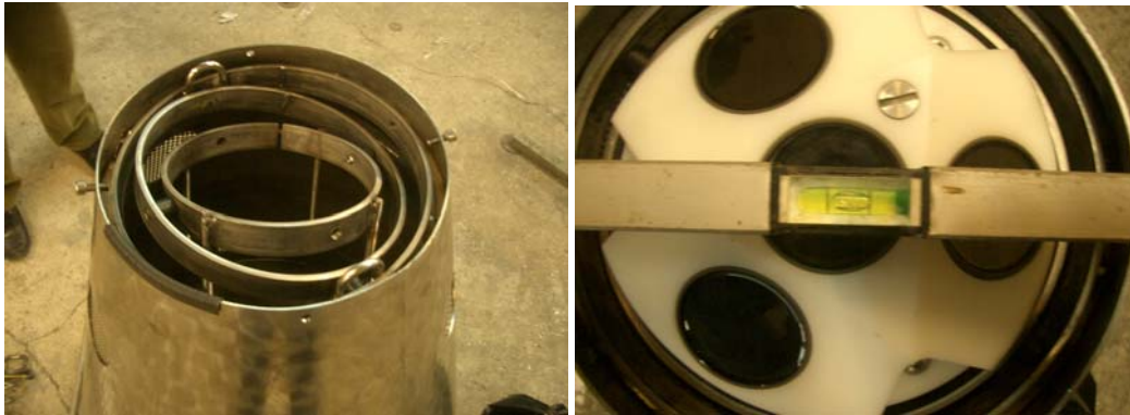
Figure 3.13. Gyroscopic ring system holding the device in vertical position
