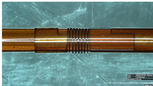
Figure 2.5 A combination of cylindrical and surface shadow mask prepared using a 4 axis Nd:YAG laser-cutting system (JK 400, P.A.L.S. Laser) from thin walled polyimide tubes.
