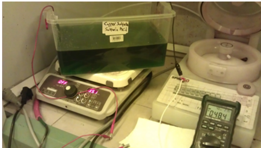
Figure 2.10 Electroplating setup including copper electroplating solution bath, heater and power supply together with multimeter for sensitive measurement of applied current.
