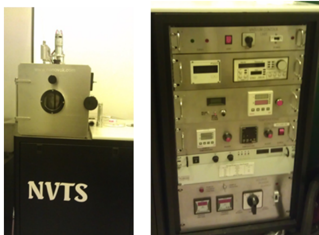
Figure 2.6 Outer view of utilized PVD thin film deposition system manufactured by NVTs, Nanovak, Turkey.
