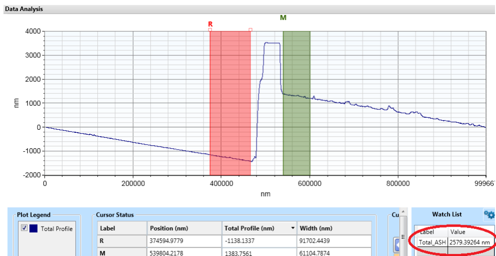
Figure 2.14 Representative measurement of the final isolating layer thickness ( 2.5 \mu\text{m} ) of Parylene C using a surface profiler (Dektak XTL, Burkert).
