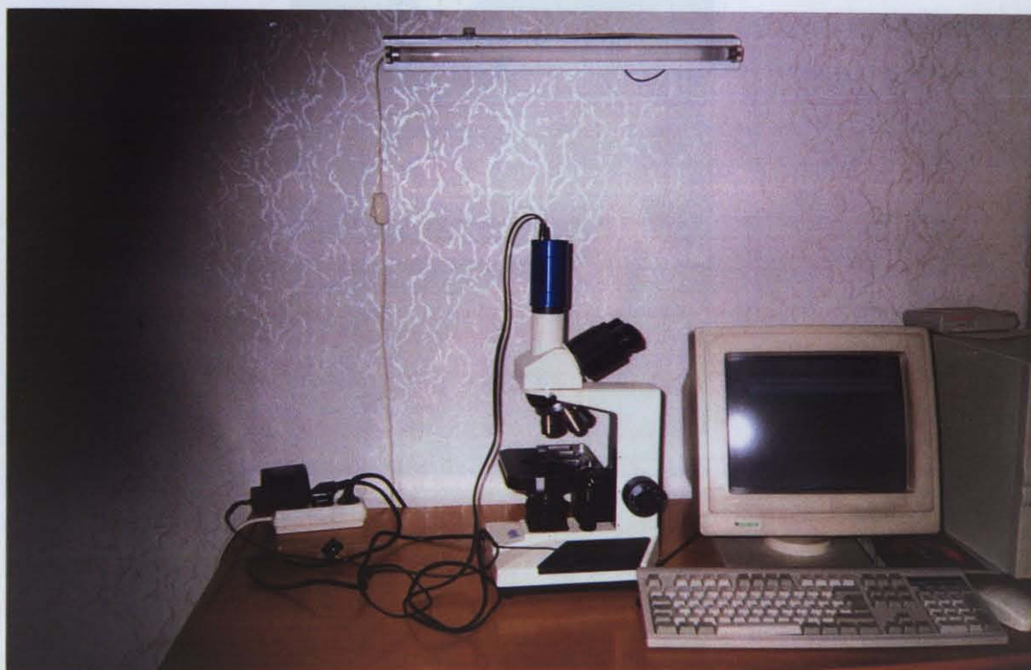
Figure 6.10 Optical, bright field microscope with digital camera attachment
