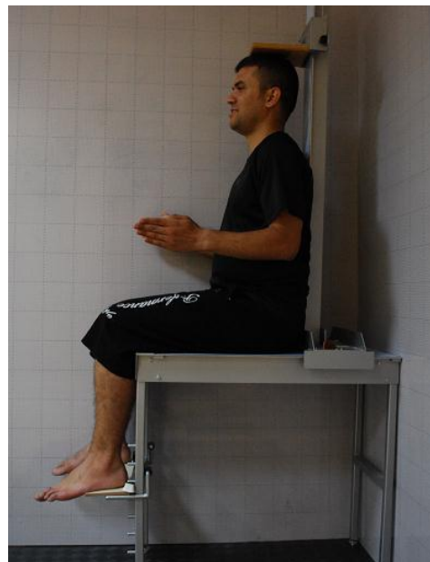
Figure 4.19. Position for the vertical dimensions in sitting obtained by sitting height table.
