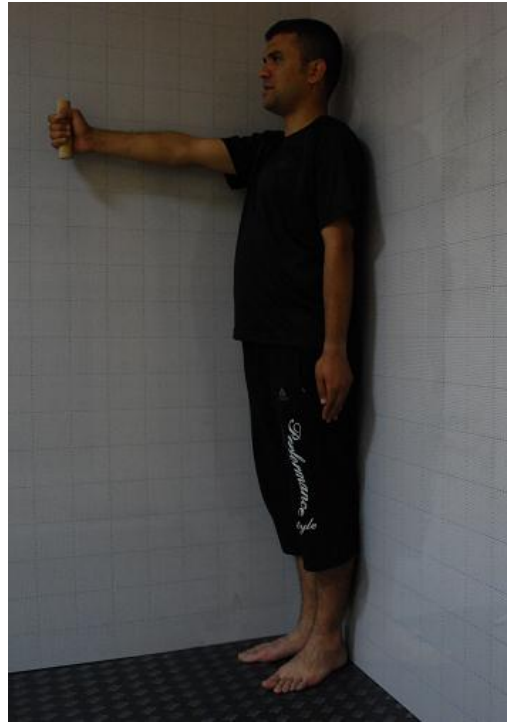
Figure 4.20. Position for the forward dimensions in standing obtained by grid board and handle diameter.
