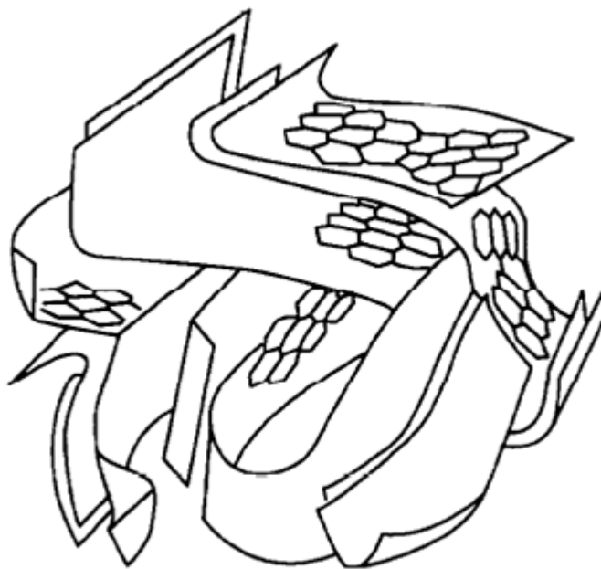
Figure 2.3. Schematic representation of the structure of activated carbon.
