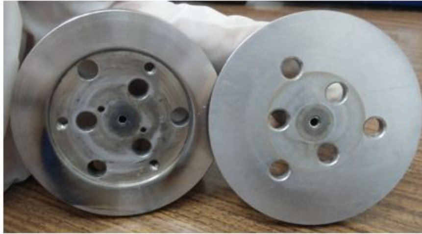
Figure 3.12. The wear on the cathode base.
