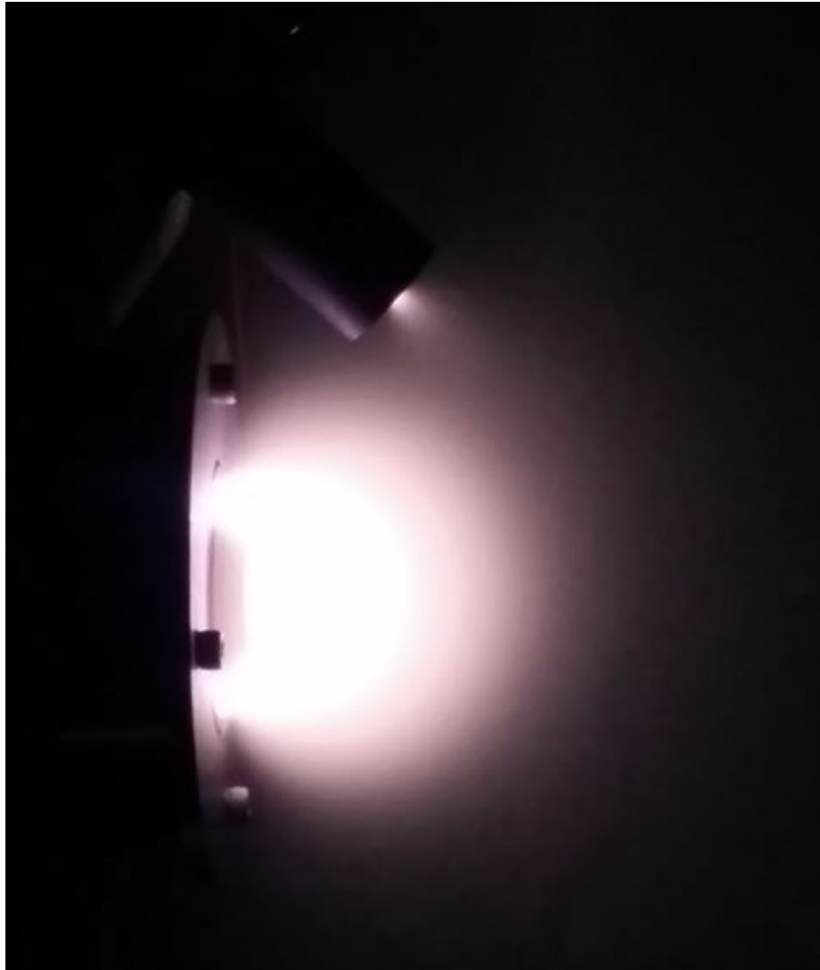
Figure 1.10. HK40 Hall effect thruster while operating inside BUSTLab vacuum chamber.
