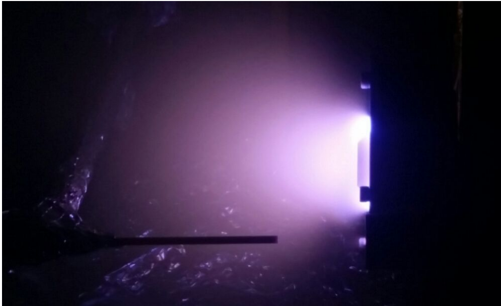
Figure 4.34. HK40 Hall effect thruster with BUSTlab LaB 6 hollow cathode.
