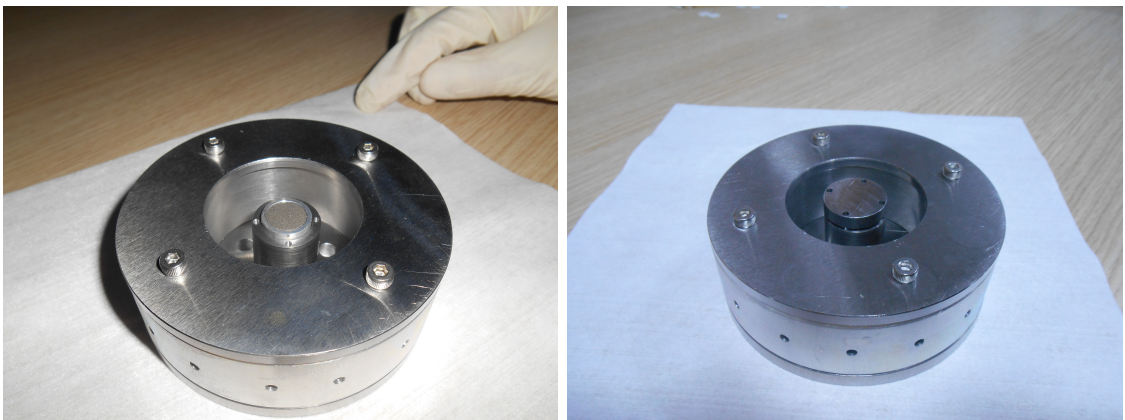
Figure 2.13. The magnet and the cap inside the BN channel.
