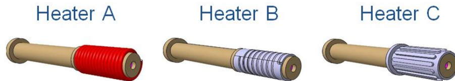
Figure 3.8. Heater A: classical heater with sheathed tantalum wire wrapped around cathode tube. Heater B: Tantalum bare wire wrapped inside helical shaped groove.
