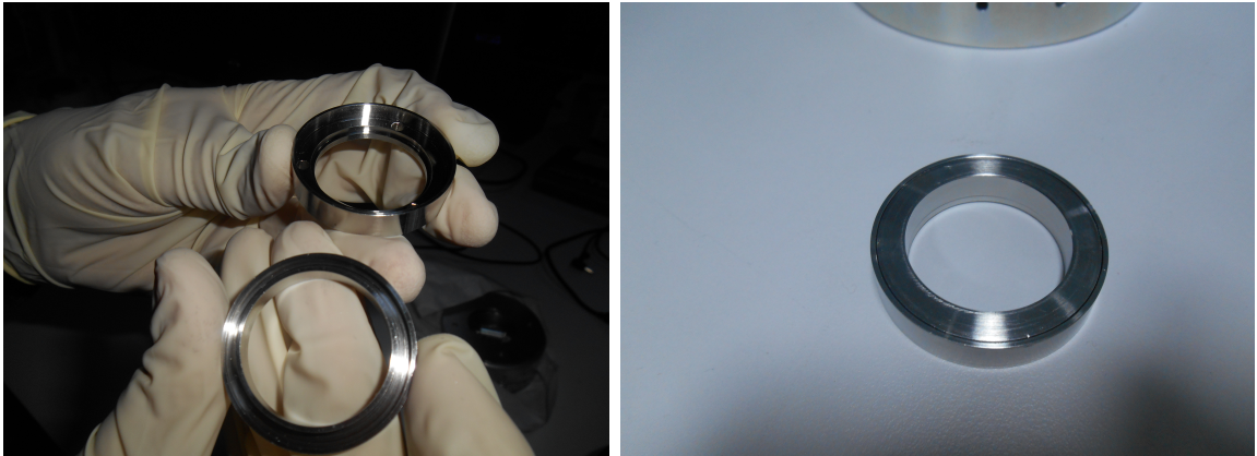
Figure 2.9. The first design of the anode and the gas distribution.
