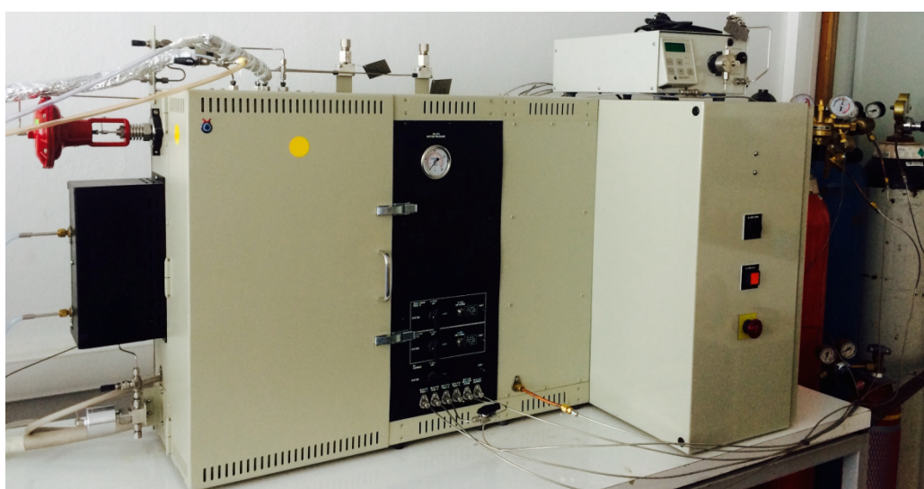
Figure 3.2. Fixed bed micro-reactor reaction system.
