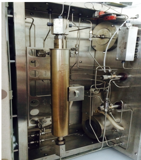
Figure 3.3. Interior oven chamber of reaction system.
