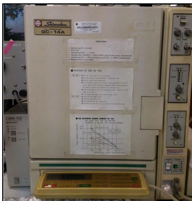
Figure 3.7. Gas Chromatography Instrument Used in the Experiments (Shimadzu GC-14A).
