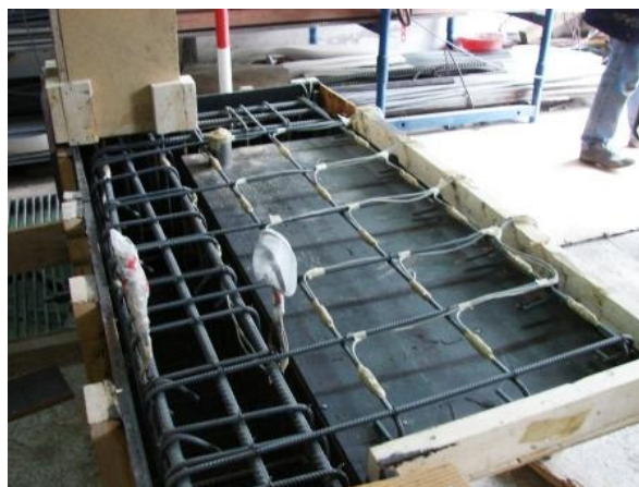
Figure 3.21. Strain gages installed in US3-CS-Control
