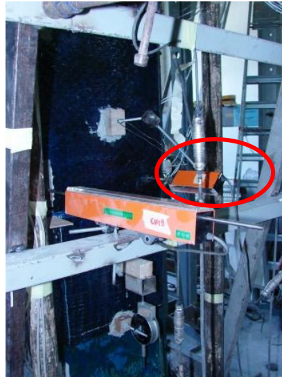
Figure 5.15. LVDT layout for slippage reading
