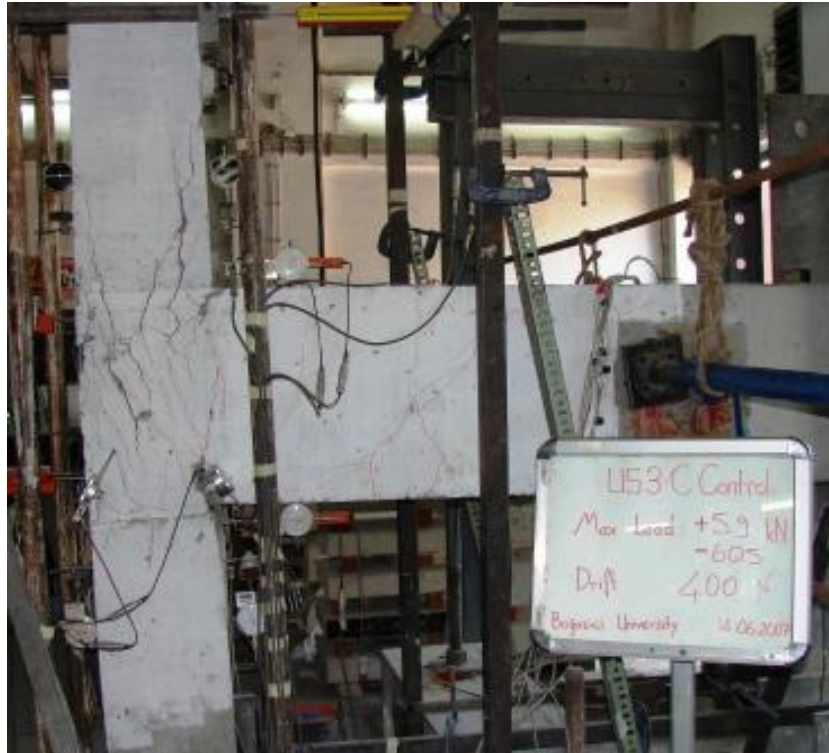
(a) Crack Pattern of US3-C-Control in pull direction of loading
