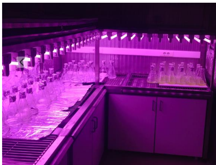
Figure 3.1. A light and temperature controlled algal culture growth chamber with continuous illumination.
