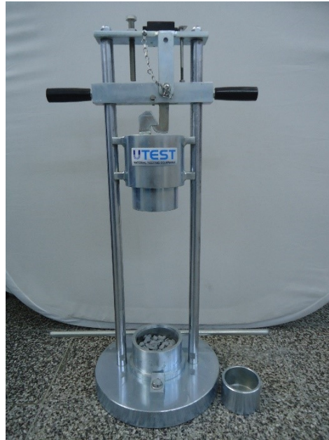
Figure 3.6. Aggregate Impact Value Test Device
