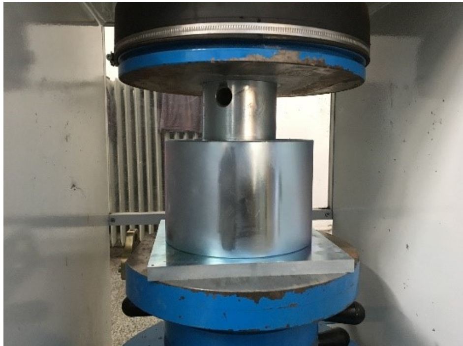
Figure 3.5. Aggregate crushing value test under compression loading
