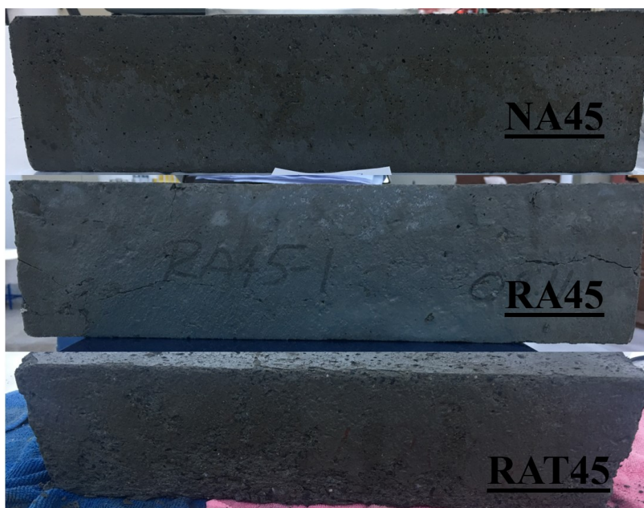
Figure 4.34. Photos of NA45, RA45 and RAT45 specimens after subjected to 126 cycles.
