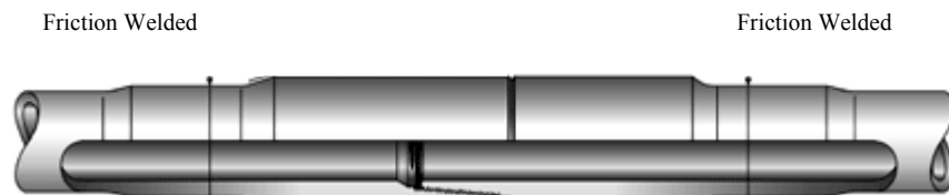
Figure 2.18 Friction welding example: drill pipes [31]
