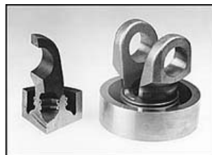
Figure 2.17. Friction welding example: diesel engine piston [11]
