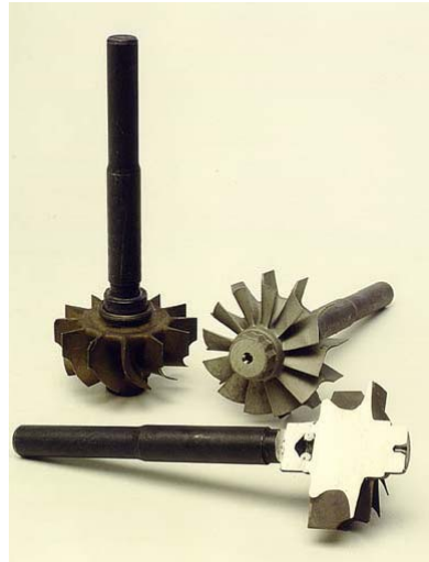
Figure 2.19. Friction welding example: turbocharger [26]
