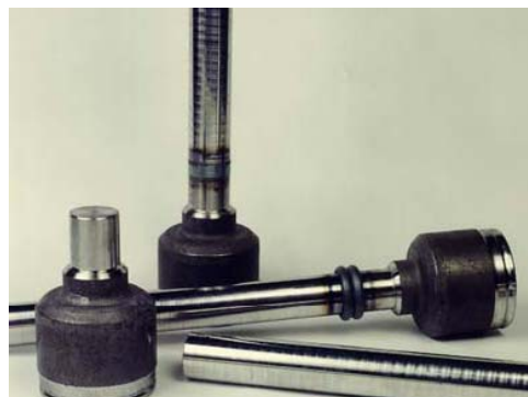
Figure 2.13. Friction welding example: drive shafts [26]
