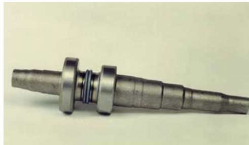
Figure 2.14. Friction welding example: gearbox shaft [26]
