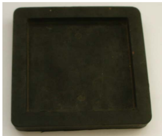
Figure 4.5. Damper for reducing vibrations
