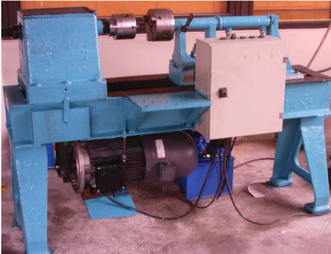
Figure 4.4. Experimental set-up built for the friction welding operation
