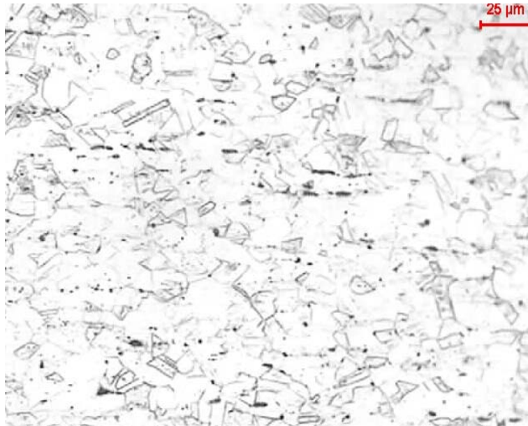
Figure 5.91. F6-AISI 304-base metal
