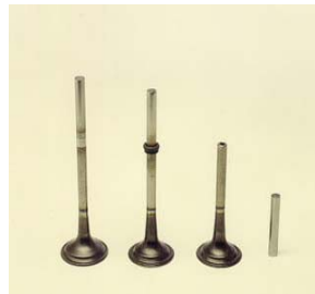
Figure 2.12. Friction welding example: exhaust valves [26]
