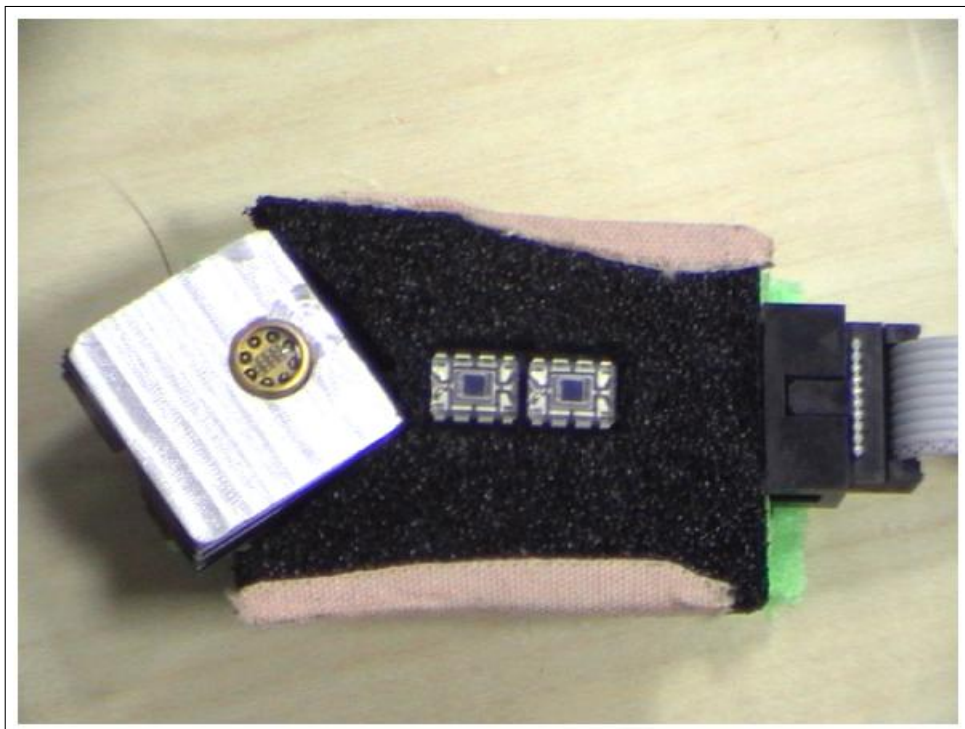
Figure 4.26 The probe used for measurements, (A) the led, (B) The detectors (C) the cooler.
