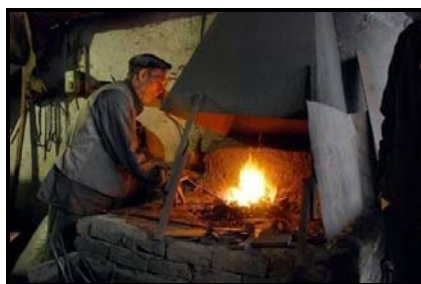
Figure 5.45. Heating of the bloom
