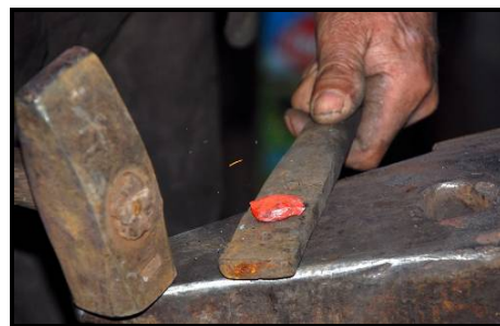
Figure 5.50. Formation of nail head
