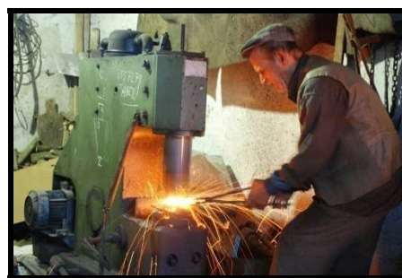
Figure 5.46. Forging the bloom
