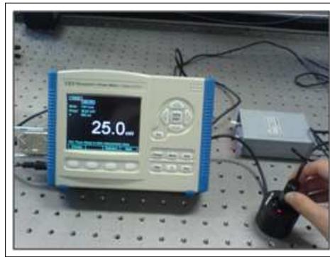
Figure 3.2 The measurement of laser power with a detector
