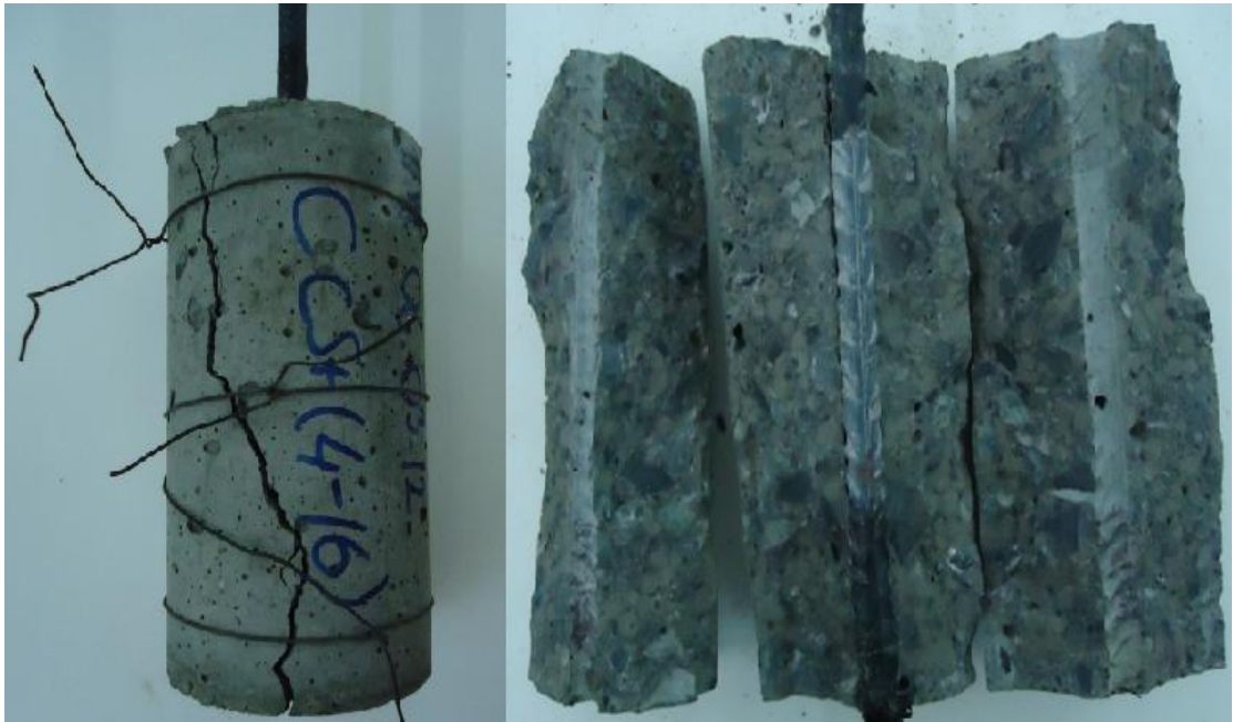
Figure B.5. Failure of pullout test specimen without tire chips.
