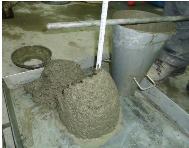
Figure 4.2. Shear slump occurring in fresh concrete with tire chips.
