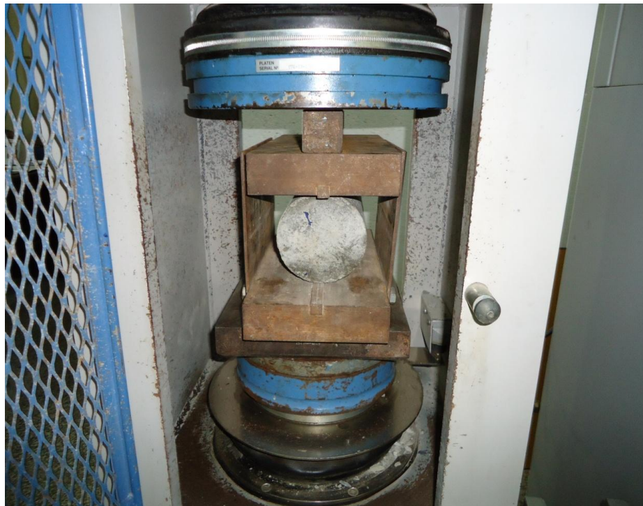
Figure 3.9. Splitting tensile strength test.
