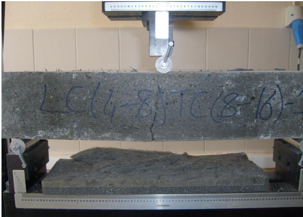
Figure B.8. Failure of three point bending specimen with tire chips.
