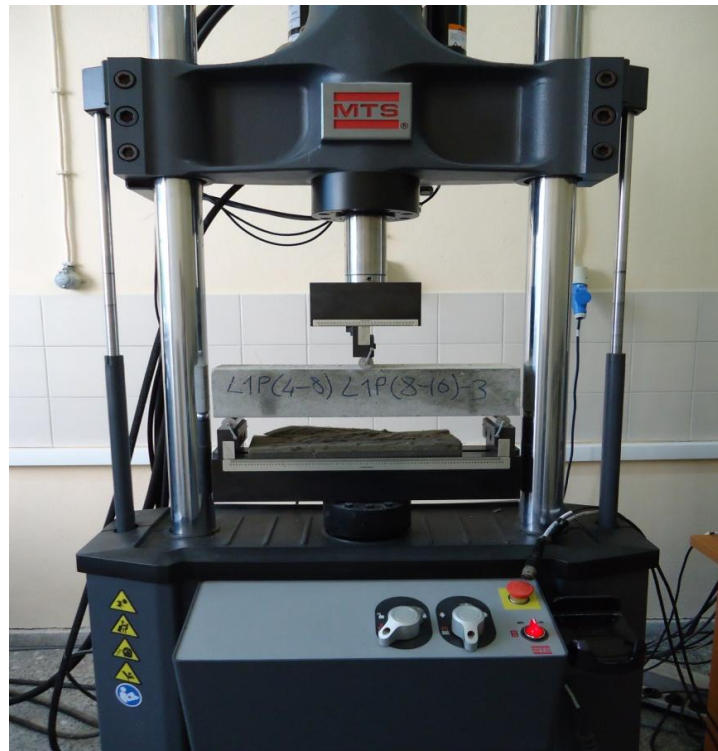
Figure A.6. Three point bending test setup.
