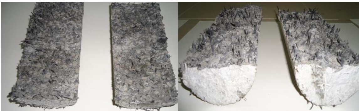
Figure 4.9. Splitting section view of specimens with LWA(4-8mm) and tire chips(8-16mm) as coarse aggregate.
