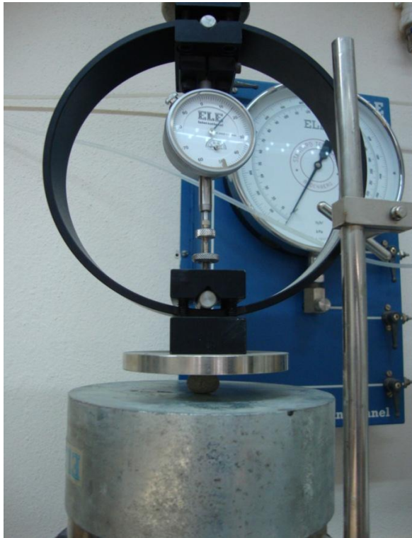
Figure A.3. Crushing setup of an individual pellet.
