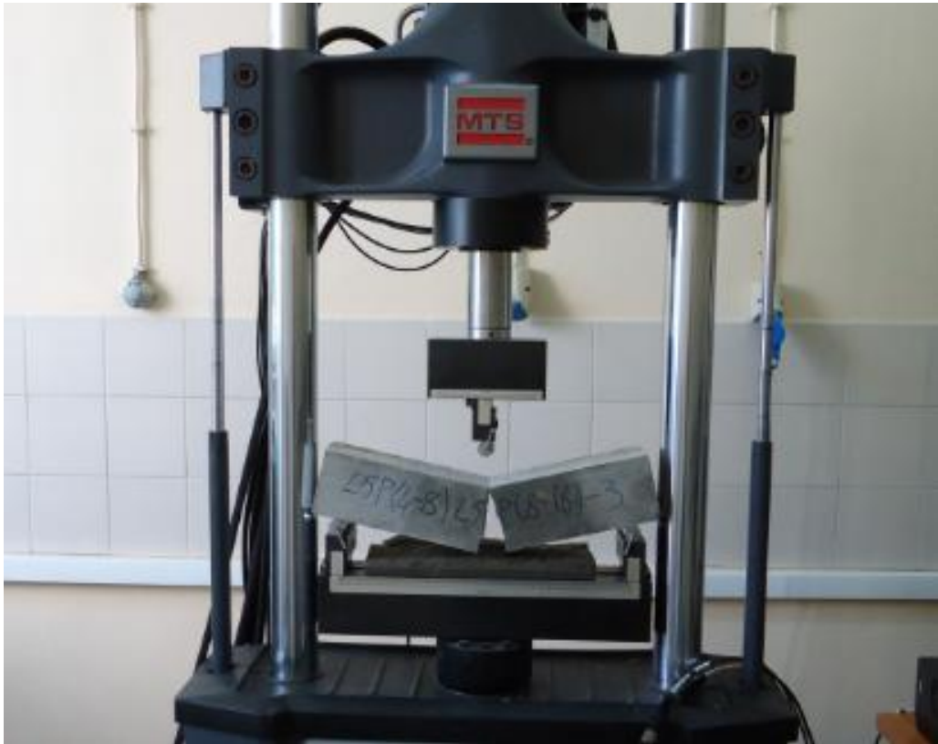
Figure B.7. Failure of three point bending specimen without tire chips.
