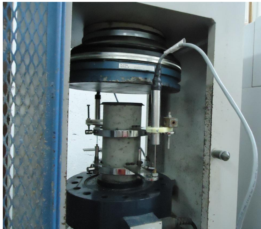
Figure 3.8. Compressive strength and modulus of elasticity test.
