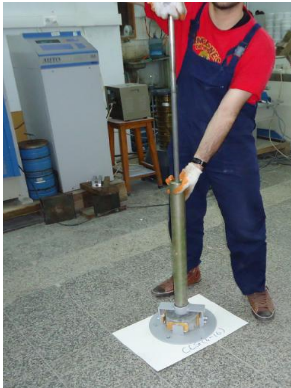
Figure A.4. Drop-weight impact resistance test setup.
