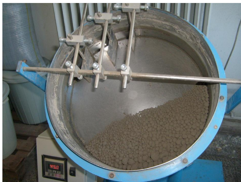
Figure A.2. Lightweight aggregate pelletization process.
