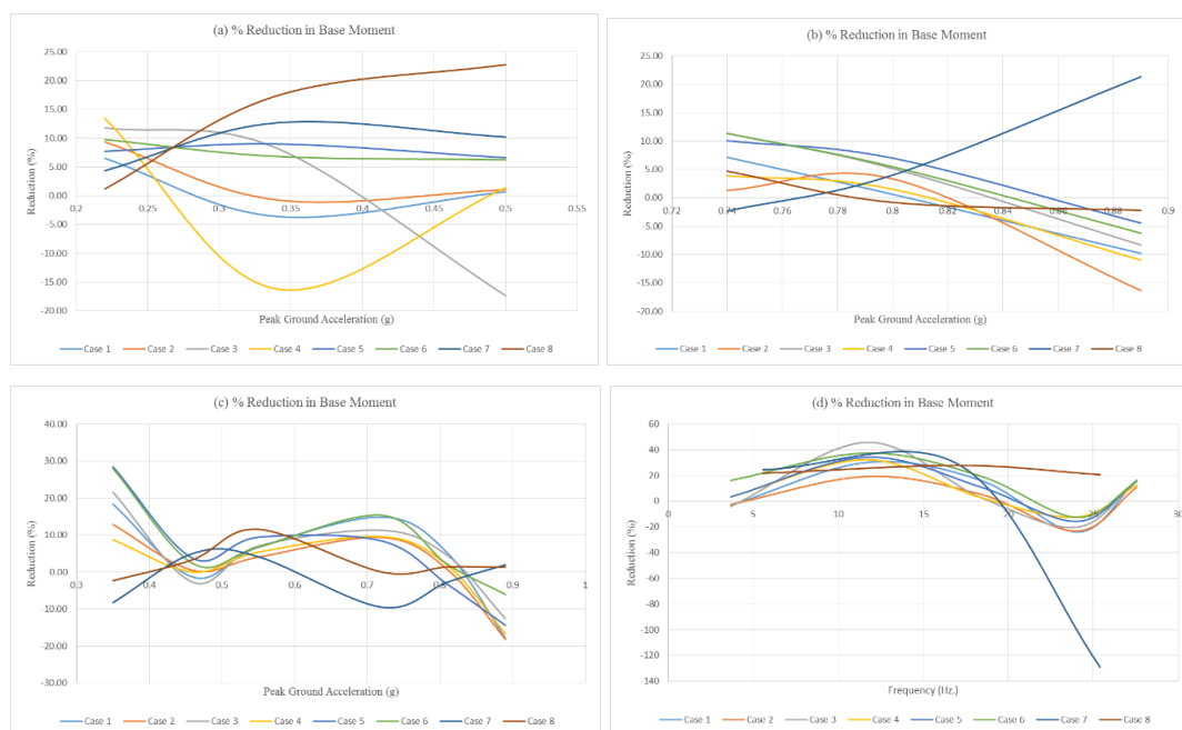
Figure 5.15. Reduction in Base Moment under (a) Kocaeli Earthquake, (b) Kobe Earthquake, (c) El Centro Earthquake, (d) Cyclic Sinusodial Motion for GSI-CL.
