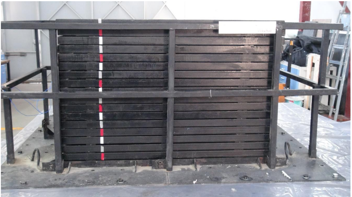
Figure 3.3. Side View of Unidirectional Laminar Box.
