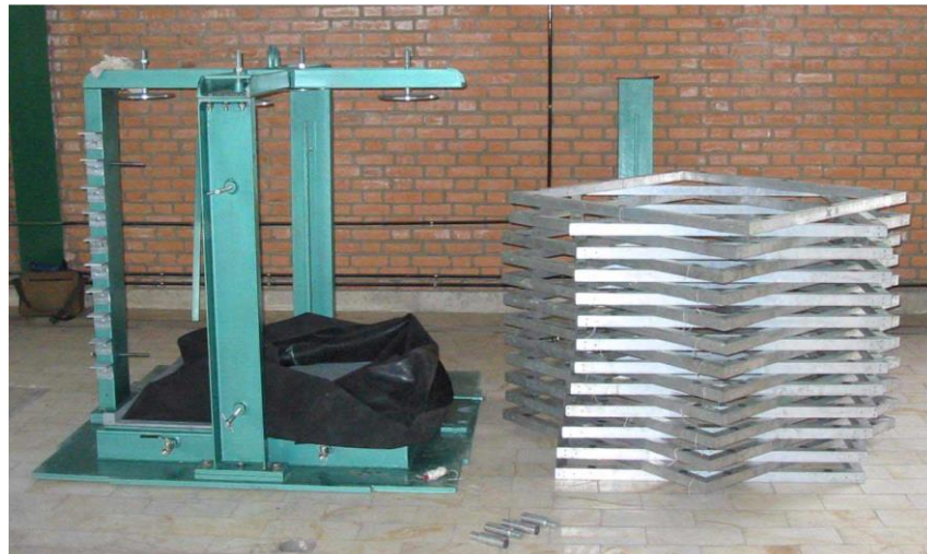
Figure 2.66. Disassembled Parts of A Laminar Box (Jafarzadeh, 2004).
