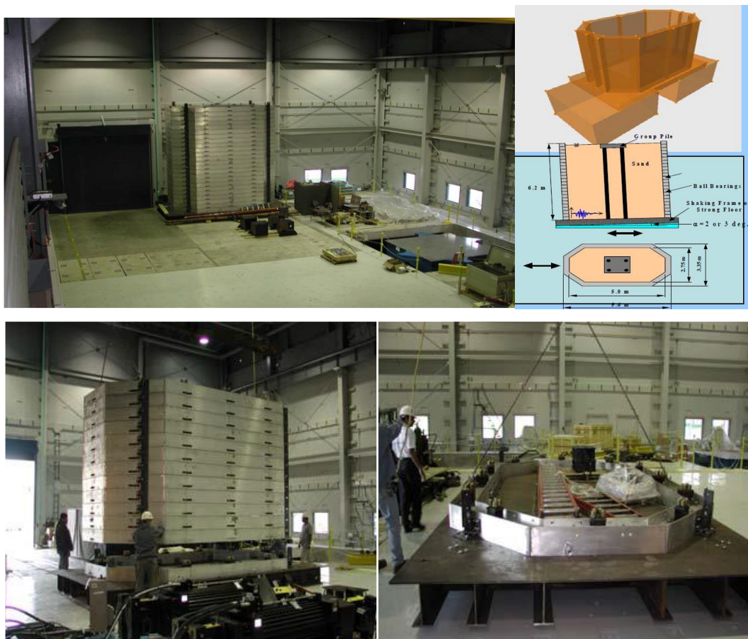
Figure 2.68. Laminar Box on Shaking Table (Thevanayagam and Ecemis, 2006).
