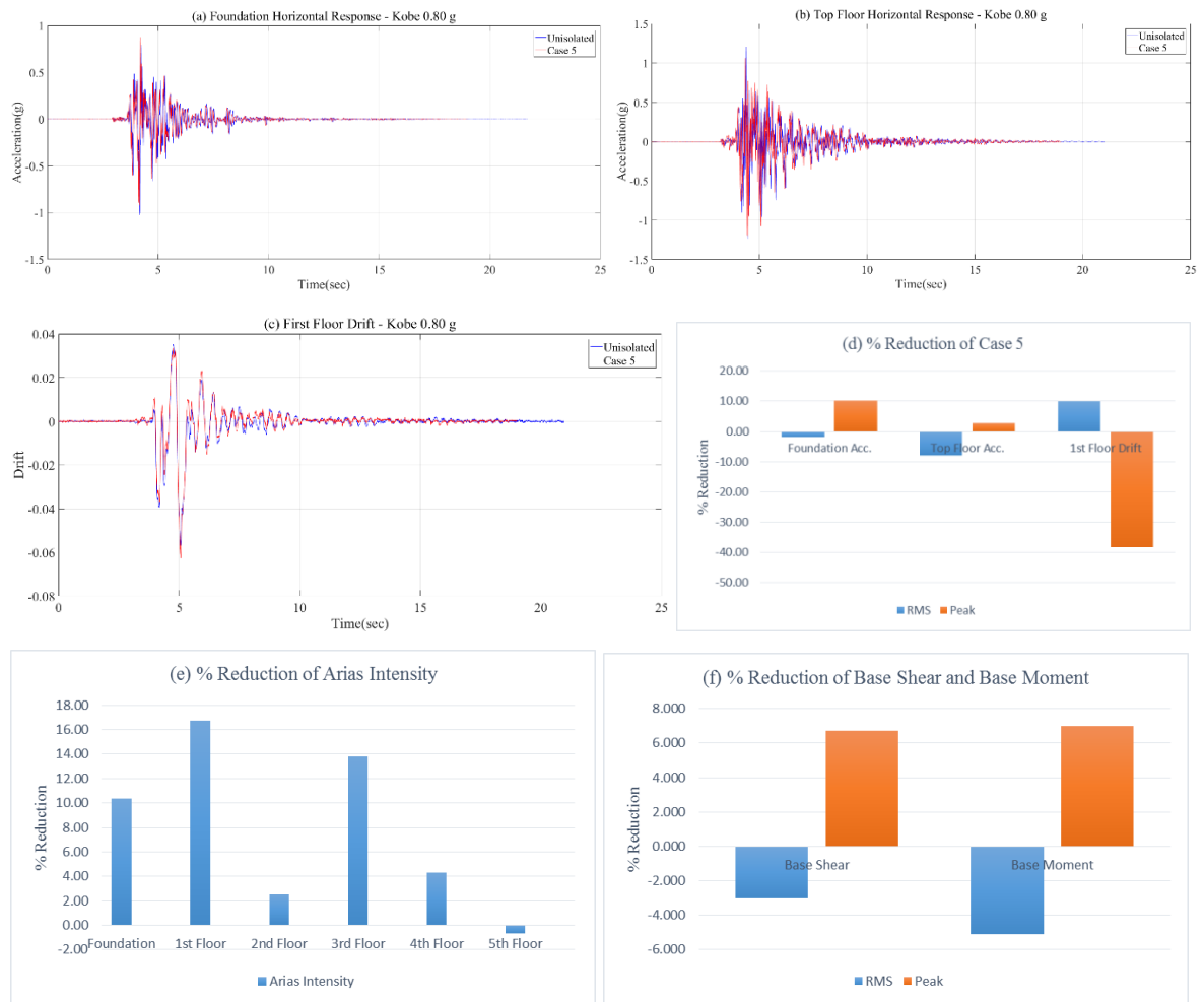
Figure 4.17. (a) Foundation Acceleration Response, (b) Top Floor Acceleration Response, (c) First Floor Drift Response, (d) % Reduction of Case 5, (e) % Reduction of Arias Intensity, (f) % Reduction of Base Shear and Base Moment under Kobe Earthquake.
