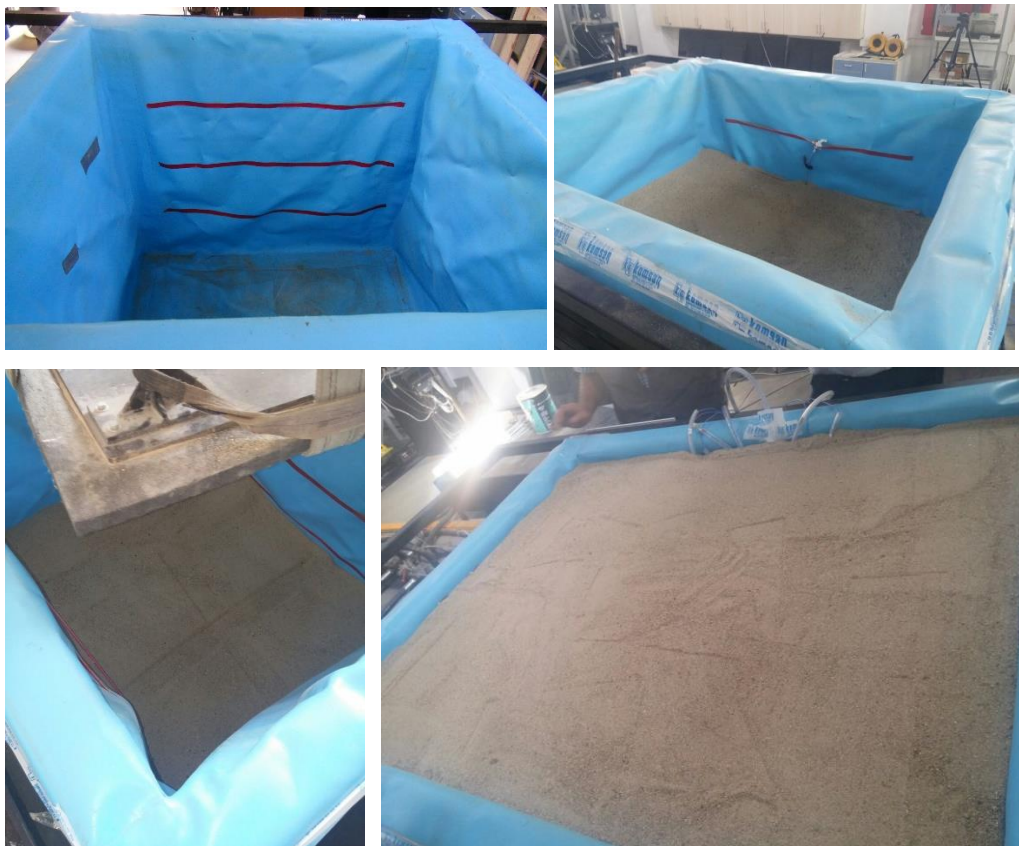
Figure 3.15. Soil Sample Preparation and Compaction.
