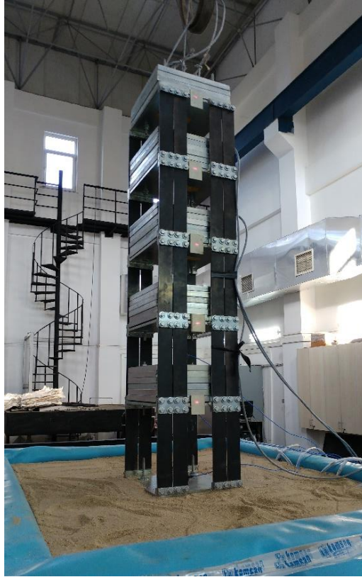
Figure 3.8. 1:10 Scaled Model of Five Story Building Model.
