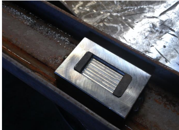
Figure 2.71. View of Roller Bearing House with Rubber Strip Stopper (Sekman, 2016; Goztepe, 2016).
