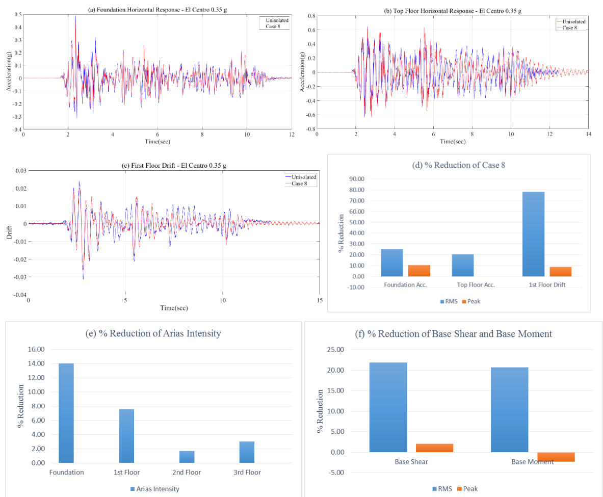
Figure 4.30. (a) Foundation Acceleration Response, (b) Top Floor Acceleration Response, (c) First Floor Drift Response, (d) % Reduction of Case 8, (e) % Reduction of Arias Intensity, (f) % Reduction of Base Shear and Base Moment under under El Centro Earthquake.
