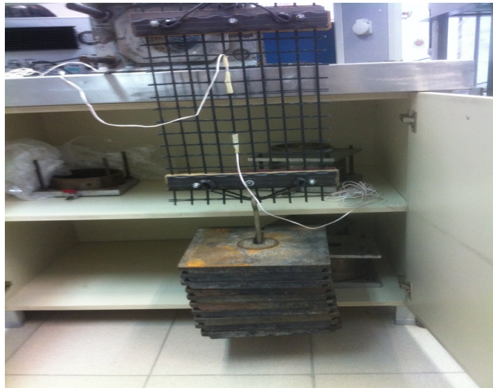
Figure 4.31. View of the Strain Calibration Test Setup.
