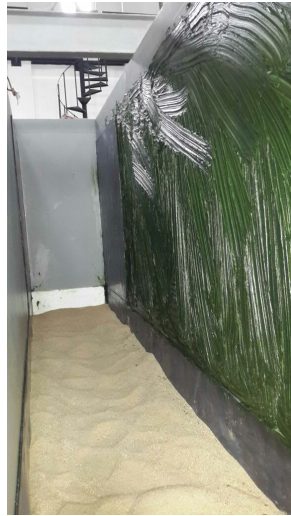
Figure 3.19. Half Full Container with Dry Sand with Grease Behind Rubber Sheet.
