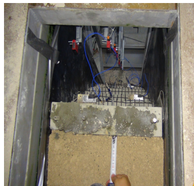
Figure 3.22. Grouted Top Blocks.
