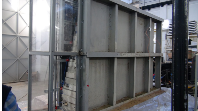
Figure 3.2. Steel Container Box with Glass Covered Frame Fixed on Shaking Table.
