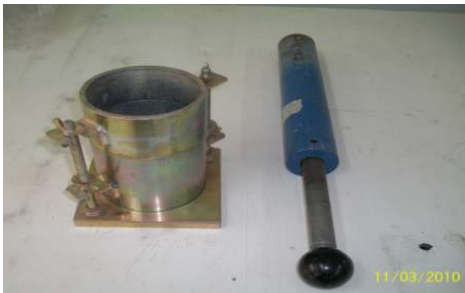
Figure 6.9. Compaction Mold and Hammer.
