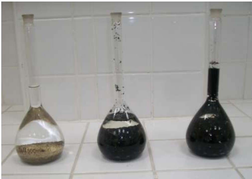
Figure 6.12. Volumetric flask with sand-water, tire crumbs-water and tire buffings-water mixtures.
