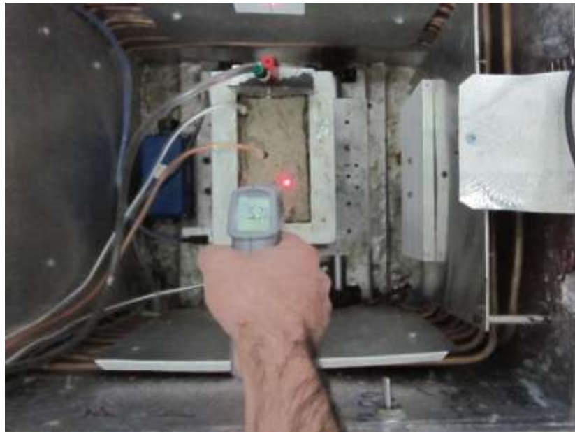
Figure 7.145. Only Sand Specimen tested at 50°C.
