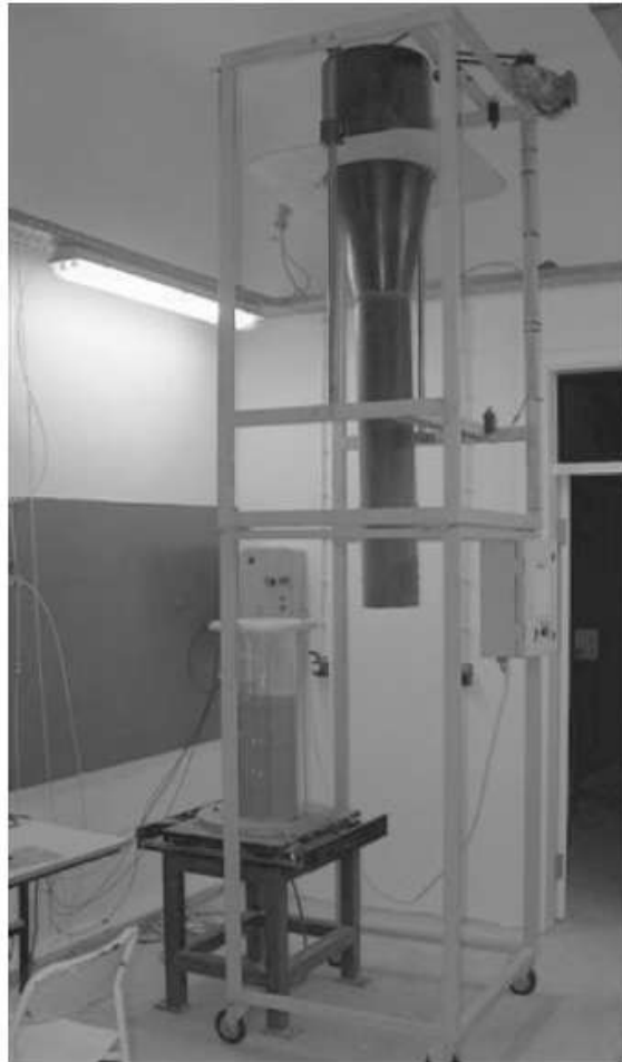
Figure 4.8. Sand pluviation system and model sand column seated on shaking table (Özener et al. , 2009).
