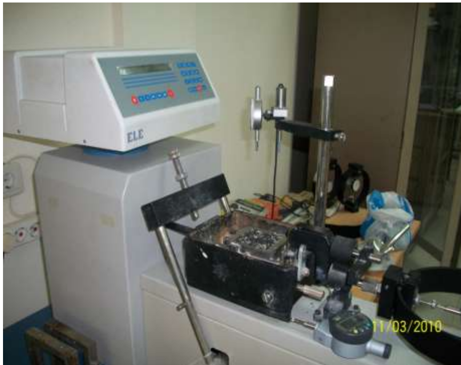
Figure 7.20. 20% tire buffings-sand specimen tested in direct shear test machine.
