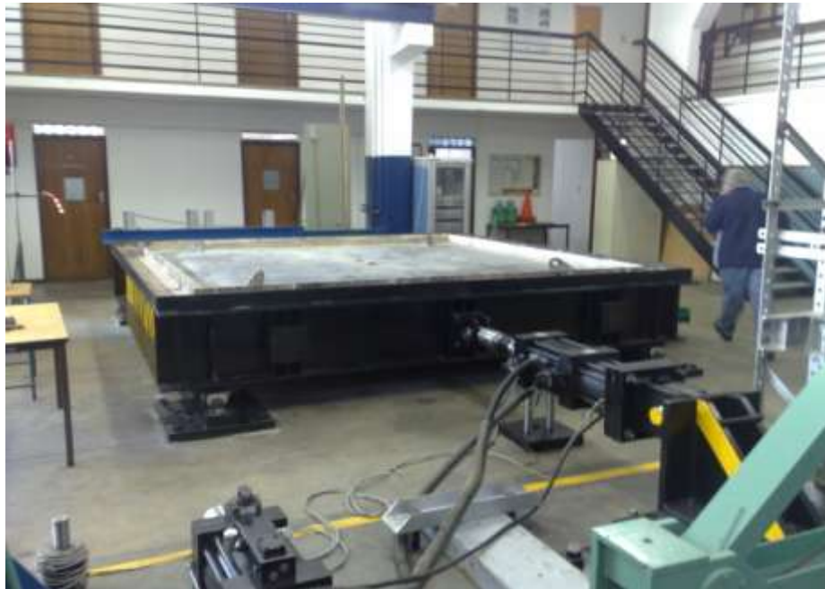
Figure 5.4. Shaking Table Test Machine.
