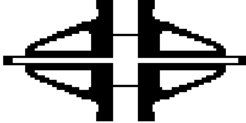
Figure 6.9. The topologically optimized inertial amplification mechanism. ( \omega_2/\omega_1 = 6.07 ).
