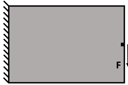
Figure 7.14. Static topology optimization problem of cantilever beam with a point load applied at the middle of the right edge.
