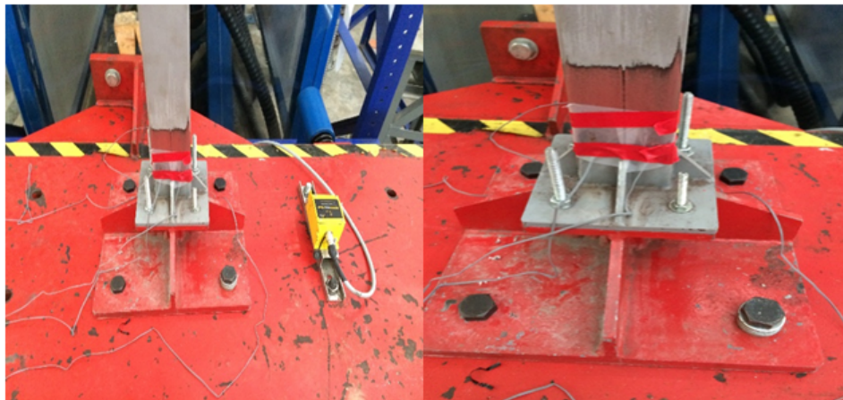
Figure 4.4. Strain gauges placement on the specimen.
