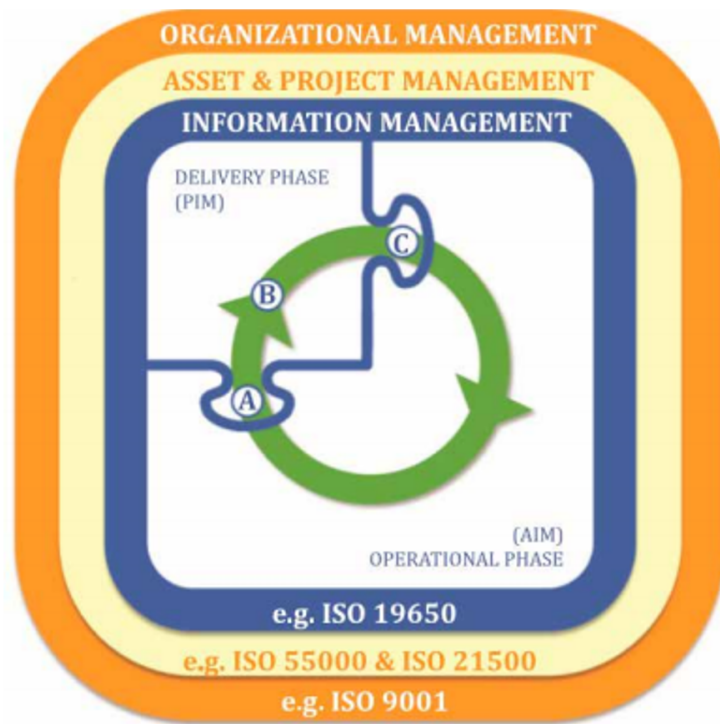
Figure 2.16. Information management lifecycle as it relates to ISO standards, according to ISO 19650.
