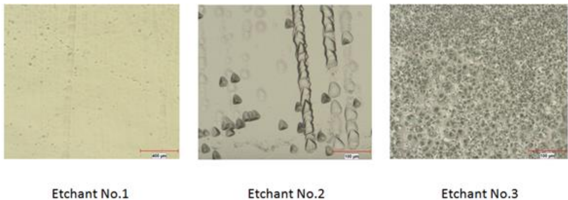
Figure 2.15. Visualization of dislocations with different etchants.
