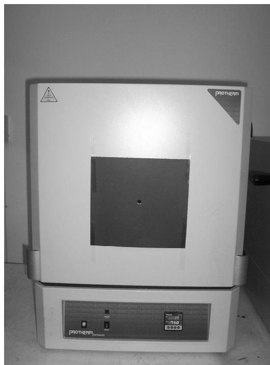
Figure 3.6. Furnace used in heat treatments of \text{TiH}_2
