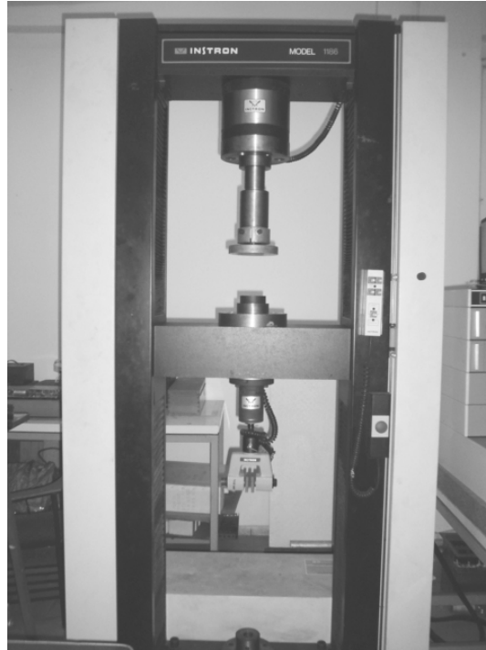
Figure 3.8. Instron test machine used in compression tests of aluminum foams
