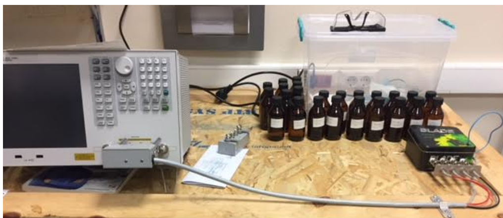
Figure 3.2 Impedance Analyzer and shielded electrode measurement box.
