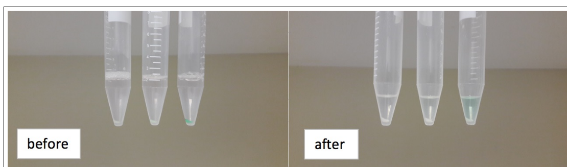
Figure 3.9 The pictures of the centrifuge tubes before and after the successful ICG extraction.
