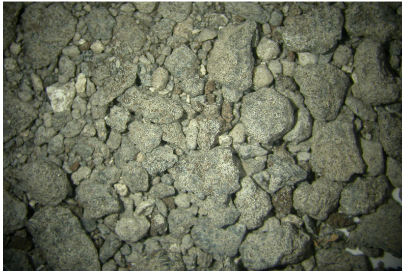
Figure 3.2. Optical macrograph of No.1 slag. (2.25 X).
