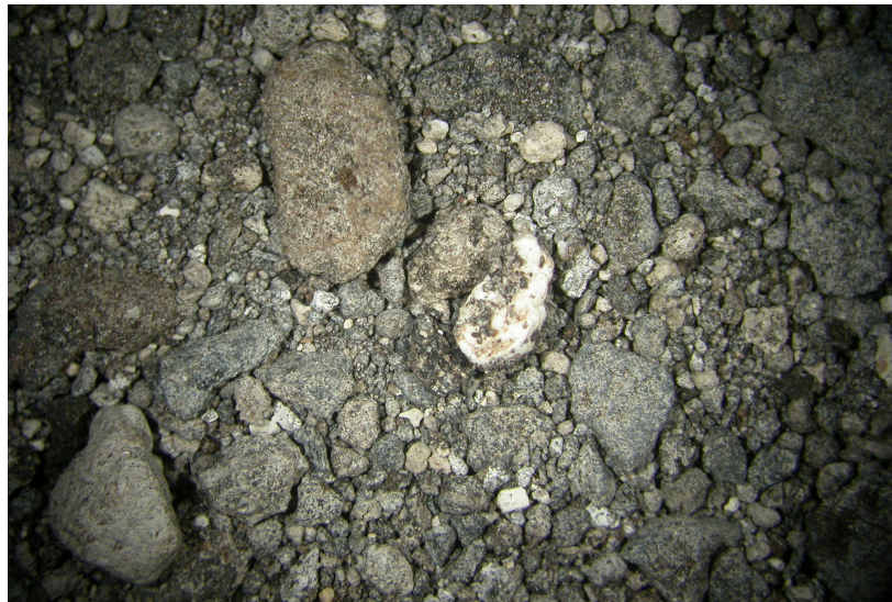
Figure 3.4. Optical macrograph of No.3* slag (2.25X).
