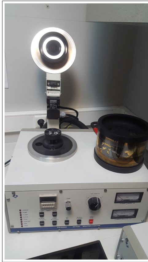
Figure 2.10 Platinum sputtering before SEM.
