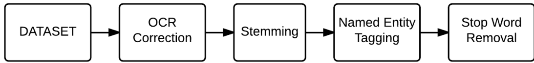
Figure 4.4. Flow diagram of the preprocessing steps.
