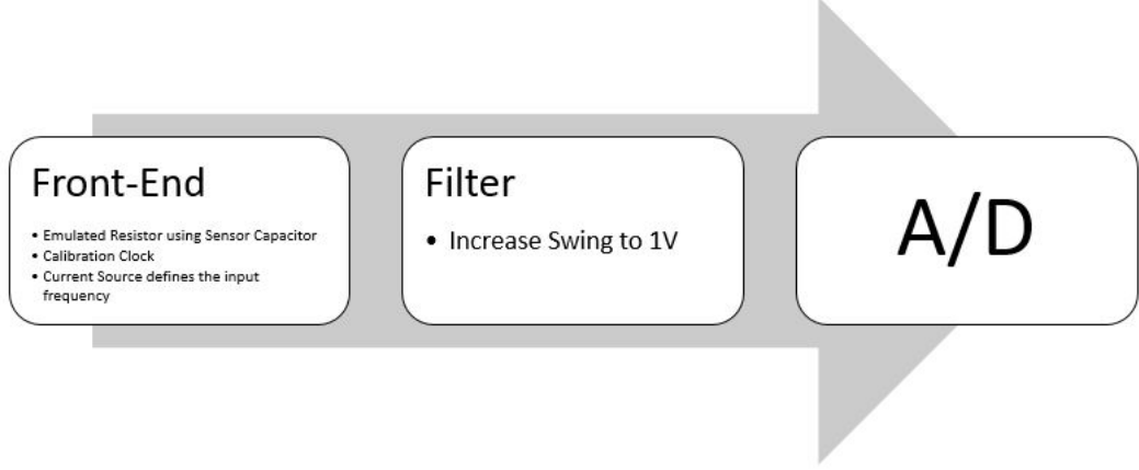
Figure 2.5. Conceptual diagram of the proposed emulated resistor based sensor interface.
